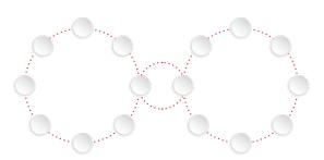
ES Net eases design and installation by supporting ring, star, bus and bridged ring network topologies. Because you can combine multiple topologies, you can create fault-tolerant, highly survivable networks while mixing and matching media between nodes to optimize cost, distances and performance.
